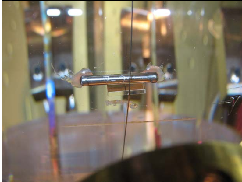
Figure 3-11. A picture of the wire placed midway along the width of the pendulum. (Photograph by Lucienne Merrill)
