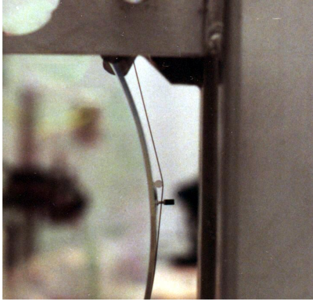
Figure 3-1. Initial LIGO standoff; a silica cylinder. The standoffs help to define the point at which the wire leaves the test mass; an attempt to improve the thermal noise in the suspensions.
