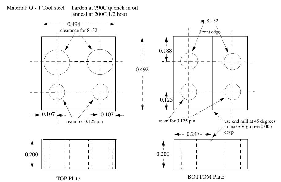
After heat treatment and cleaning, lap mating surfaces of clamp on a flat stone with 600 grit paper. Assemble clamp with pins and screw together. Lap front edge to establish a single plane with no step to hold wire.
