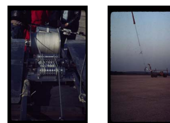
Reel with 2000 ft of nylon line to separate payload and balloon
