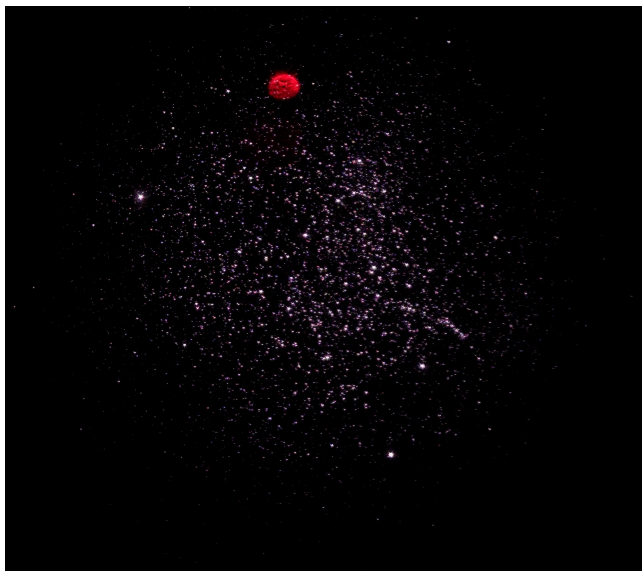
FIG. 10 (Color online) (top) Surface phase map (in units of nm) of one of the Advanced LIGO arm cavity mirrors after applying the high reflectivity mirror coatings (ZygoEPO, 2011). (bottom) infrared image of an initial LIGO arm cavity mirror taken with the cavity locked, highlighting the abundance of point defects. The red oval is the diffuse scatter from an auxiliary beam used for tracking the mirror angle.
