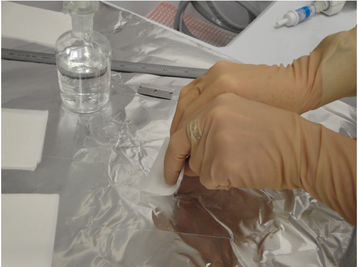
Figure 12: Contacting the wetted edge of the tissue to the surface (in this case, using the aluminum covered table as the optic surface). This image shows that the tissue bends as it adheres to the surface and the tissue is gently pulled across the surface. Again, the rings, don't wear them in a real procedure!
