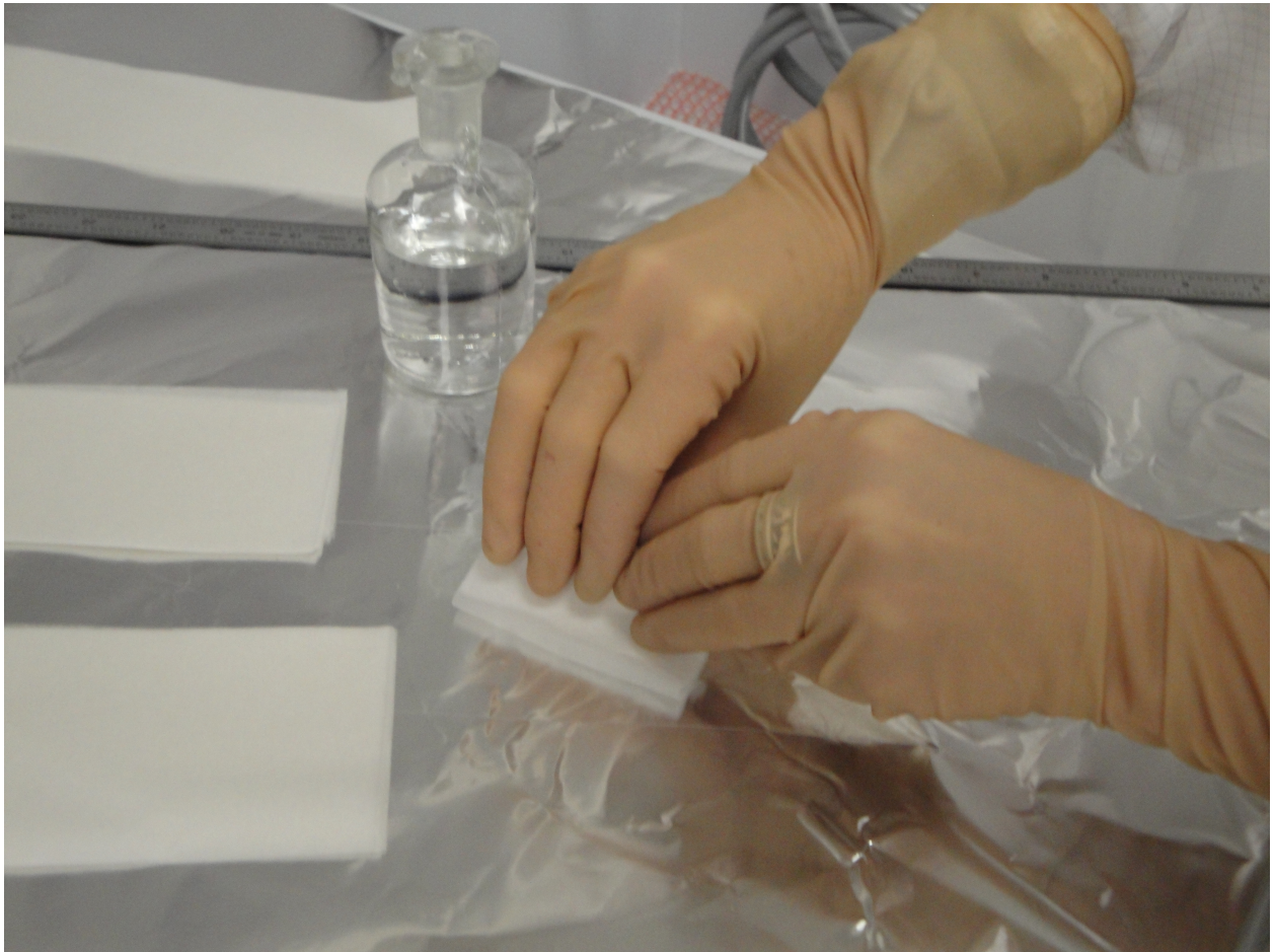
Figure 11: Contacting the wetted edge of the tissue to the surface (in this case, using the aluminum covered table as the optic surface). Note that I am wearing rings under my gloves in this demonstration picture, but they should NEVER be worn during a real cleaning procedure.
