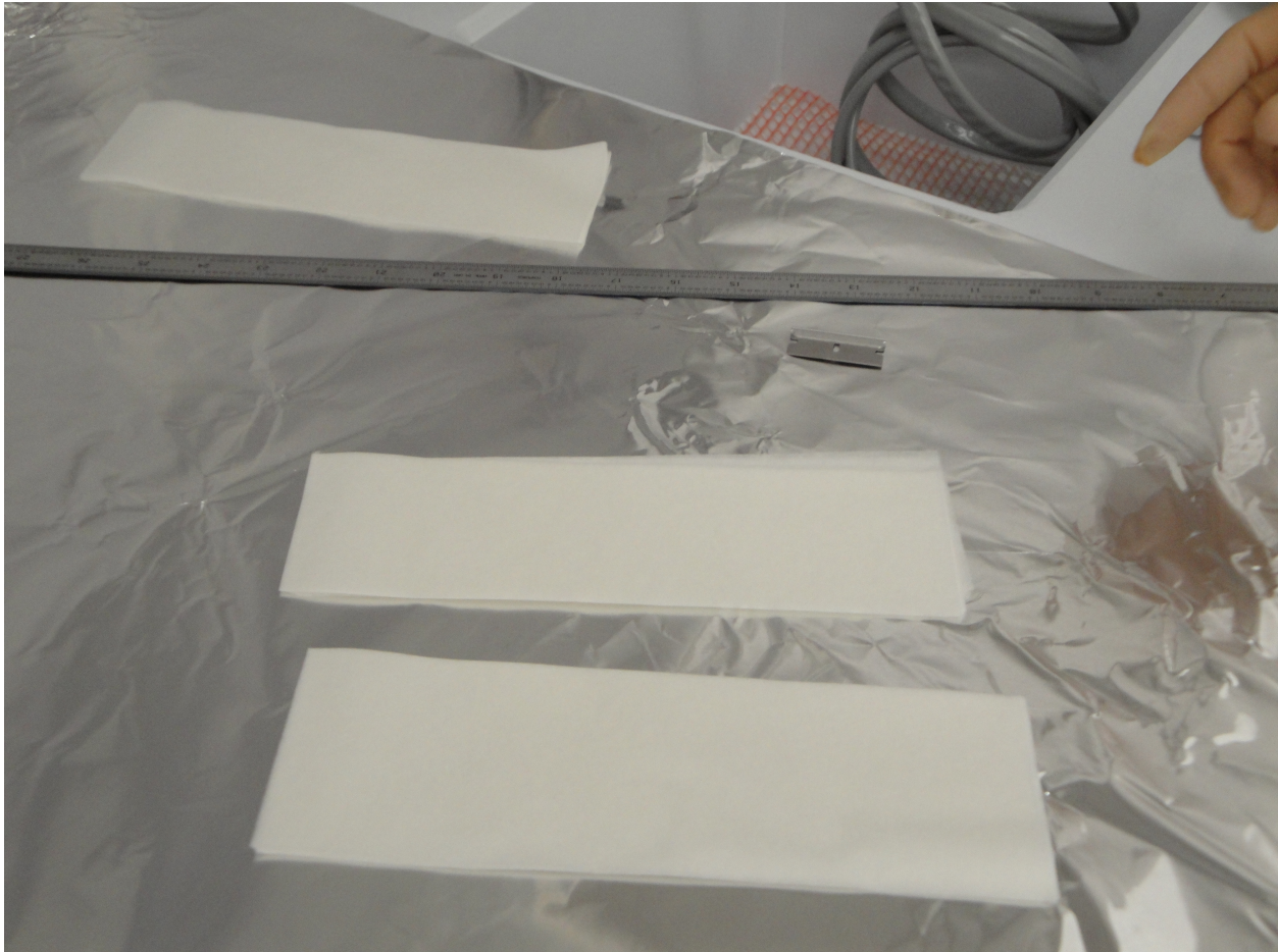
Figure 5: 9" x 9" lens tissue cut into 3" strips.
