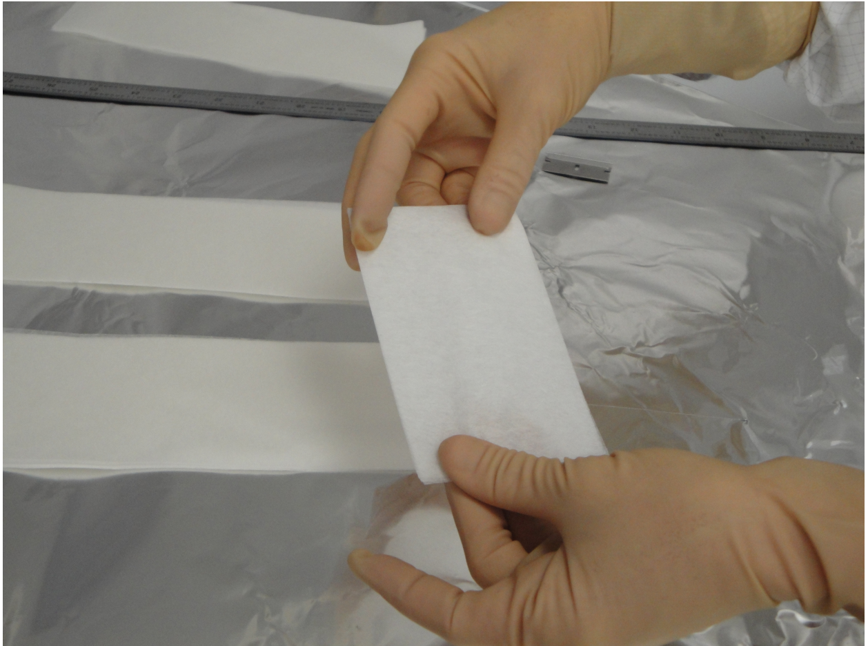
Figure 7: Lens tissue strips folded in half.
