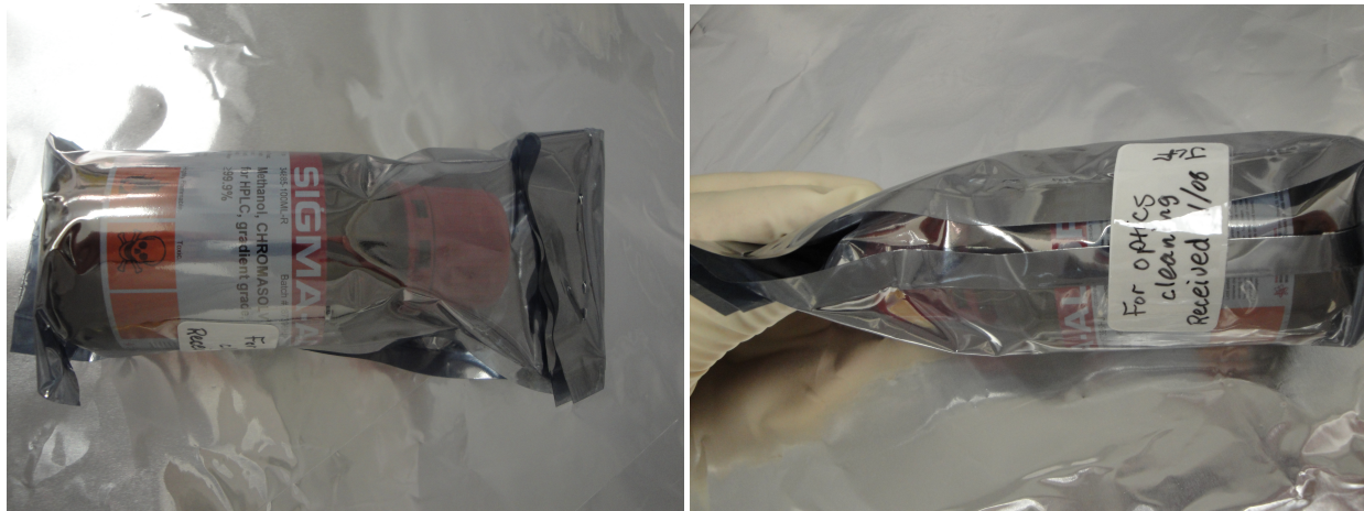
Figures 1 and 2: Chromasolv wrapped and sealed in Ameristat, to ensure that the lid's airtight seal is not broken before use.
