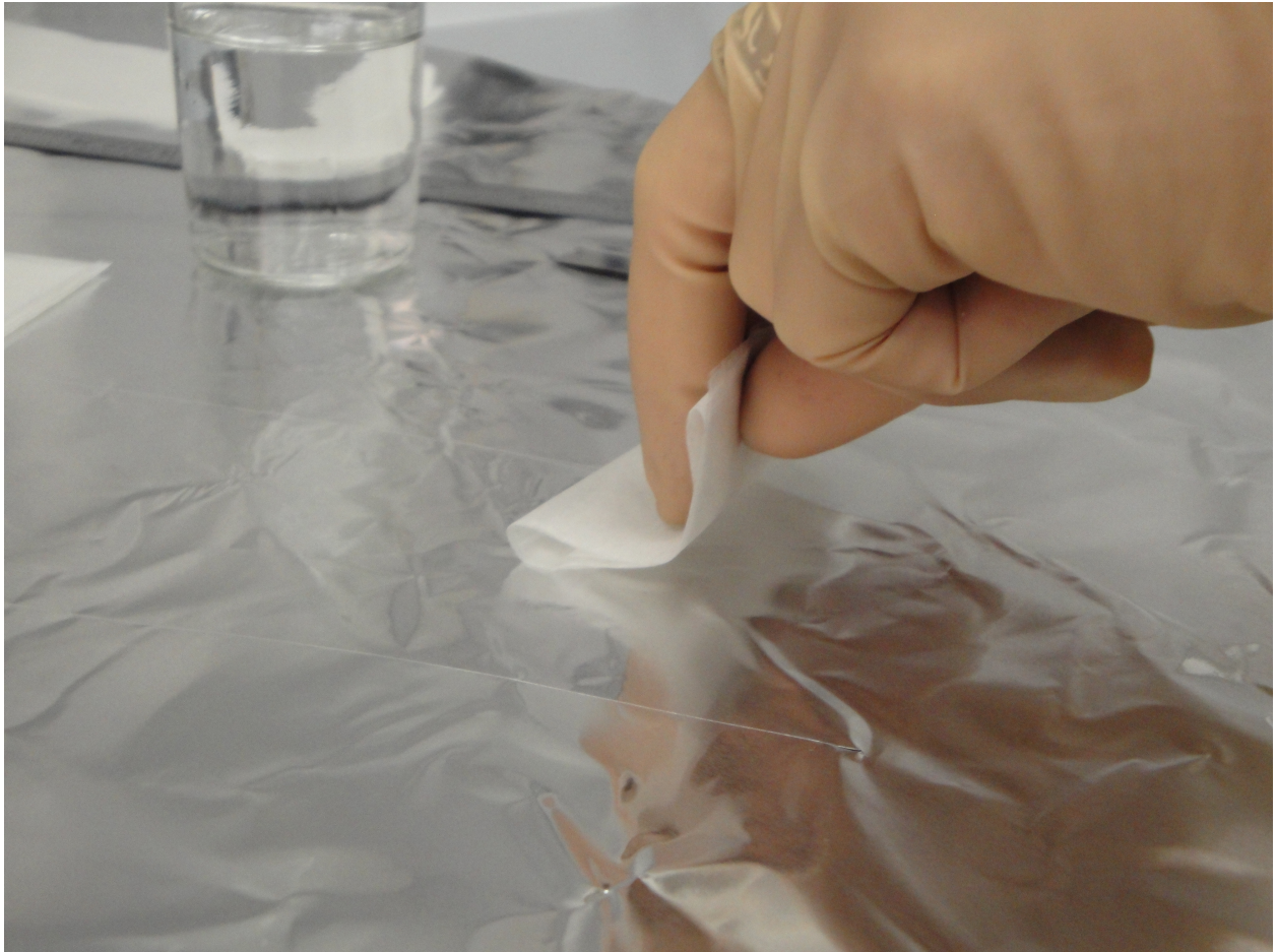
Figure 13: This shows that the only the wetted area of the tissue contacts the surface of the optic. The fingers do not contact the surface, and do not press the tissue directly onto the optic. Again, rings – don't wear them! This is just a demo picture.
