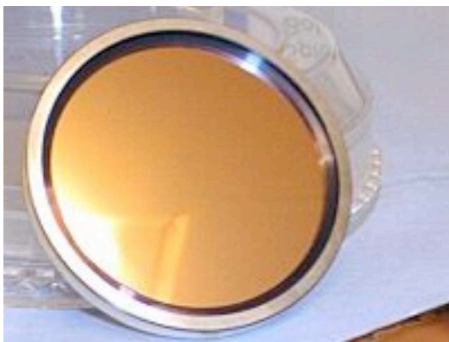
Figure 8.4: Photograph of a quasi-optical metal-mesh low-pass filter (courtesy of Peter Ade).
