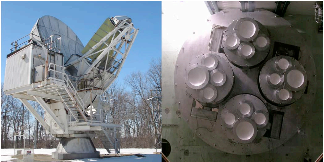
Figure 8.2: Left: Lucent 7m telescope currently used by the CAPMAP experiment measuring CMB polarization at four arc minute scales. Lucent Laboratories has offered the telescope for continued CMB research. Right: CAPMAP focal plane with its 16 radiometers in 4 cryostats. The useful part of the focal plane is more than 48” in diameter.
