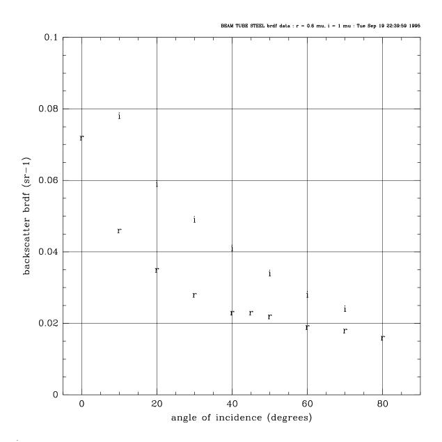
Figure 3 Backscatter brdf of the oxidized beam tube steel surface at 0.63 (r) and 1.06 (i) microns as a function of the angle of incidence.
